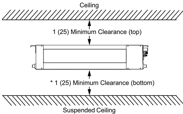
**\* NOTE - Bottom unit clearance can be 1 inch (25 mm), but allow 12 inches for filter removal on end return air applications**
